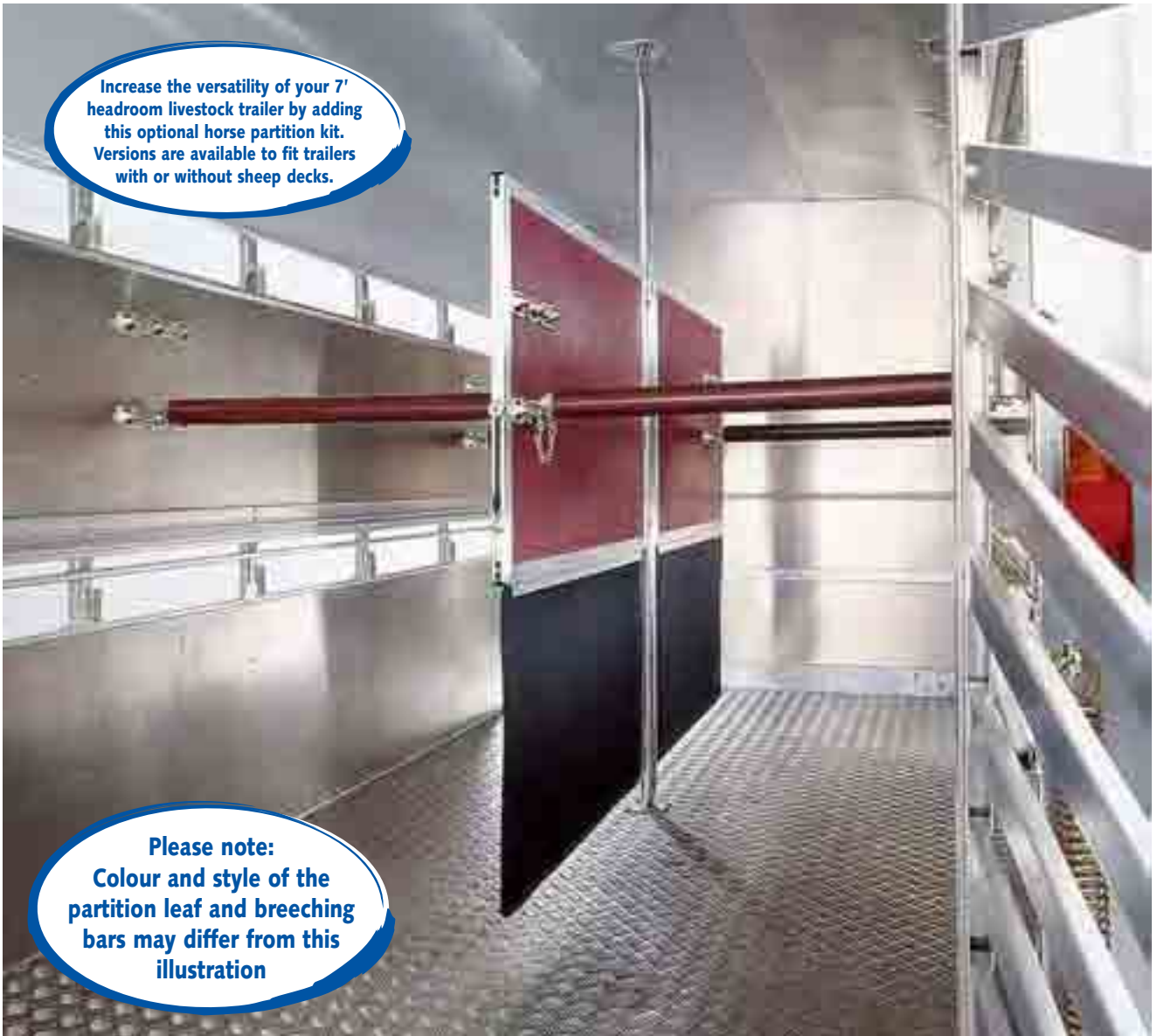
TA510 12' long 7' headroom with KX0186 horse partition kit fitted
